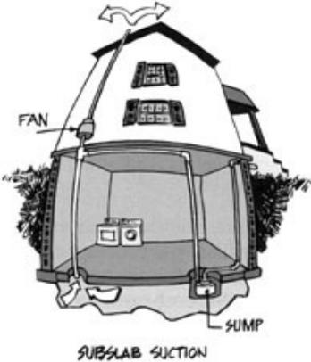
from outside the house. The number and location of suction pipes that are needed depends on how easily air can move in the crushed rock or soil under the slab, and on the strength of the radon source. Often, only a single suction point is needed.
